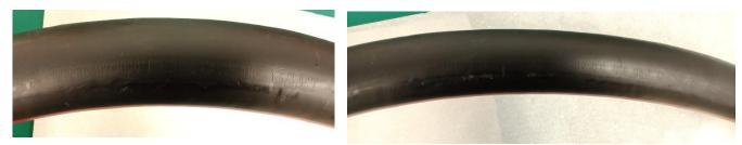
"OIPL P01516 02/2020 ELECTRIC CABLE DCF 1.5/1.5 KV 1C X 400 SQMM AL/X-90/NYLON/HDPE FOR DC USE ONLY GEN. AS/NZS 1429.1" Embossed.
