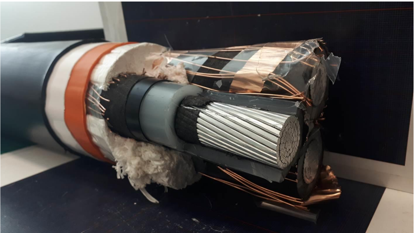
Construction of cable
